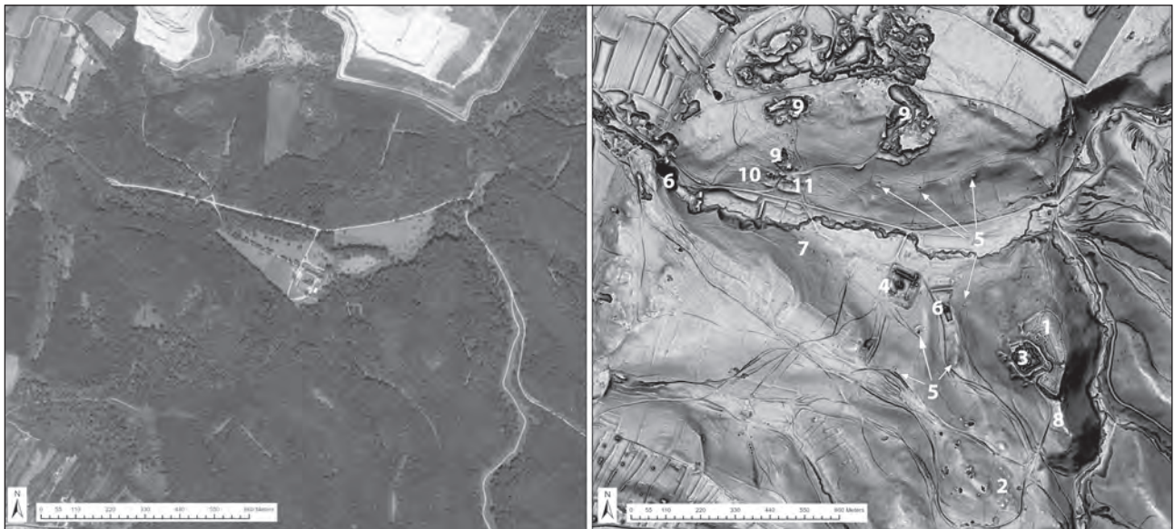
Fig. 2. Left: Orthophotograph of the case study area. The area is covered by woodland. Only the area next to the friary (centre) is clear of trees (no. 4 in right image). To the right, the remains of Scharfeneck Castle (no. 3 in right image) rise above the canopy (source: basemap.at). – Right: Ground-point filtered digital feature model of the same area based on a high-resolution airborne laser scanning data acquisition from April 2007 (visualization: combined visualization for archaeological topography). See text for description of numbers (Graphics: M. Doneus).
